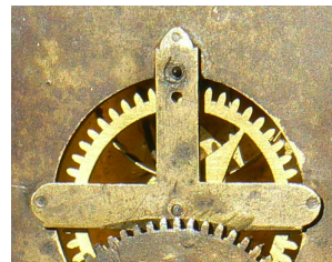
Fig. 8: "Trident" bridge on the front-plate
