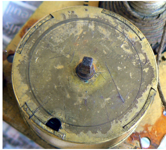
Fig. 5: Dovetailed barrel cap
