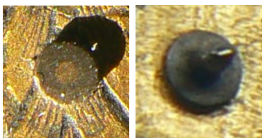
Fig. 7: Bushed pivot-holes of the verge
