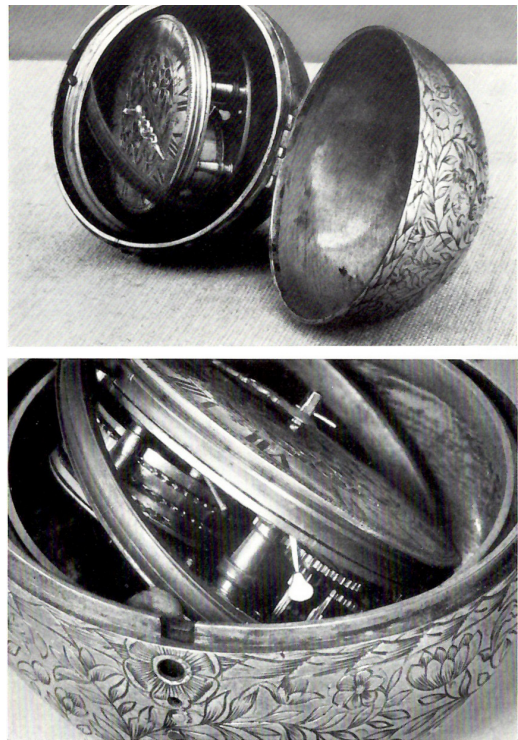
Fig. 4. Pendulum watch with a gimbal system, probably German. From von Bassermann-Jordan and von Bertele, Montres, pendules et horloges , p. 271, photographed in the Hessisches Landesmuseum, Kassel.
