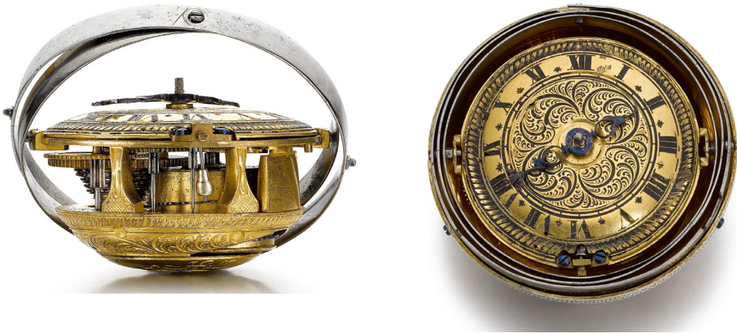
Fig. 3. Pendulum watch with a gimbal system by Mattheus Hallaÿcher, c. 1675–80. Courtesy of Sotheby's.
