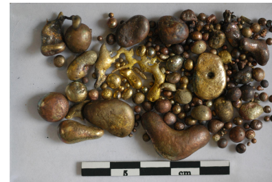
Metallic conglomerates obtained after cementation
